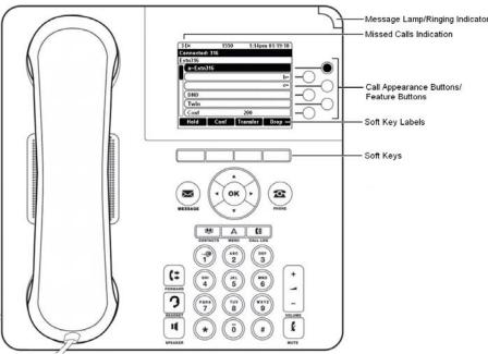
The phone supports 24 programmable call appearance/feature buttons. The labels for 6 of these are displayed in the main display and can be controlled by the adjacent buttons to the right. You can use the  $\clubsuit$  up/down  $\blacktriangledown$  keys to scroll the display. You can also use the  $\blacktriangleleft$  left/right  $\blacktriangleright$  keys to move through the button feature in pages of 6.
